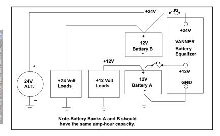
output. When a 12 volt load is present, and Battery A's voltage decreases to just below the voltage of Battery B, the battery equalizer activates and transfers sufficient current from Battery B to Battery A, satisfying the load and maintaining an equal voltage and charge in both batteries.
