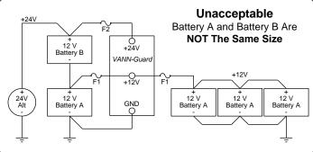
In certain applications, such as private coach or alternate energy applications, it may be desirable to have additional 12 volt "House Batteries" to operate heavy 12 volt (inverter) loads. Use the *VANN-Guard* to charge the additional batteries.
