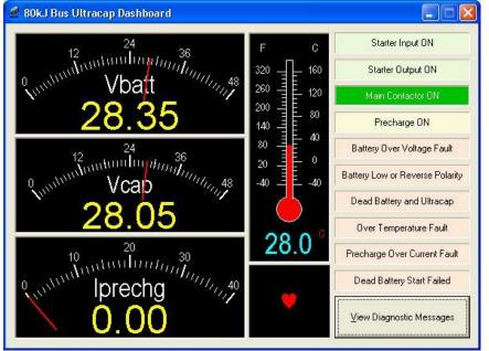
The left portion of the dashboard displays the battery and UltraCap voltages in addition to the Pre-charge current. The right portion of the dashboard illustrates status and fault messages.
