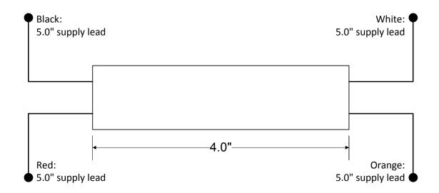
Installation Notes: The battery and switched supply inputs should both be protected with a 2A fuse.
