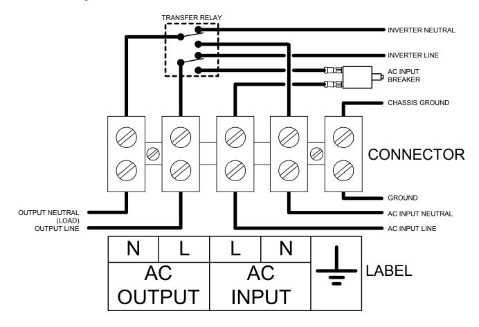
Connect AC output and AC input wiring to the VTS series terminals. Please take the following information as your reference.
