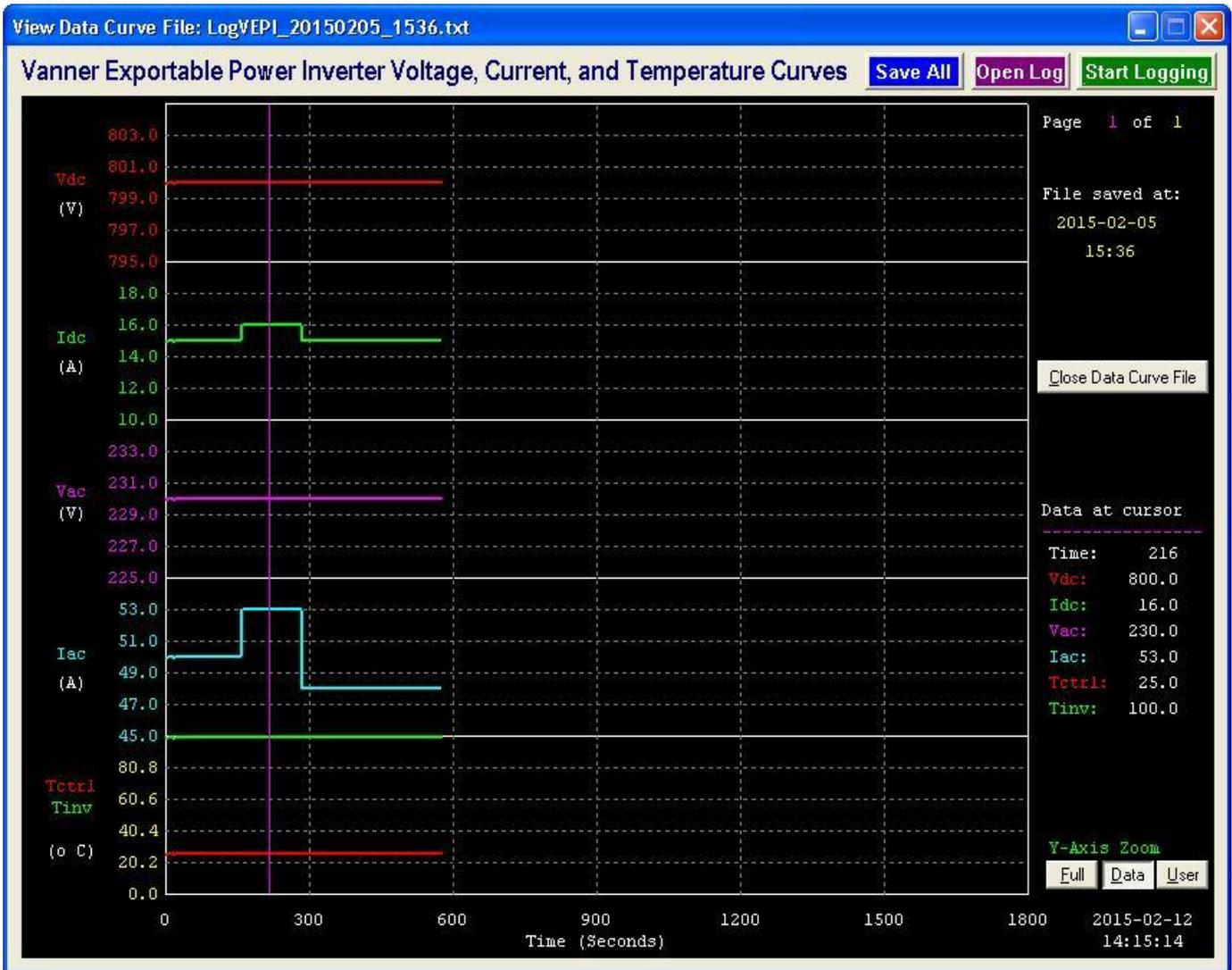
Figure 55. VEPI Data Curves Window – Open Saved Data
