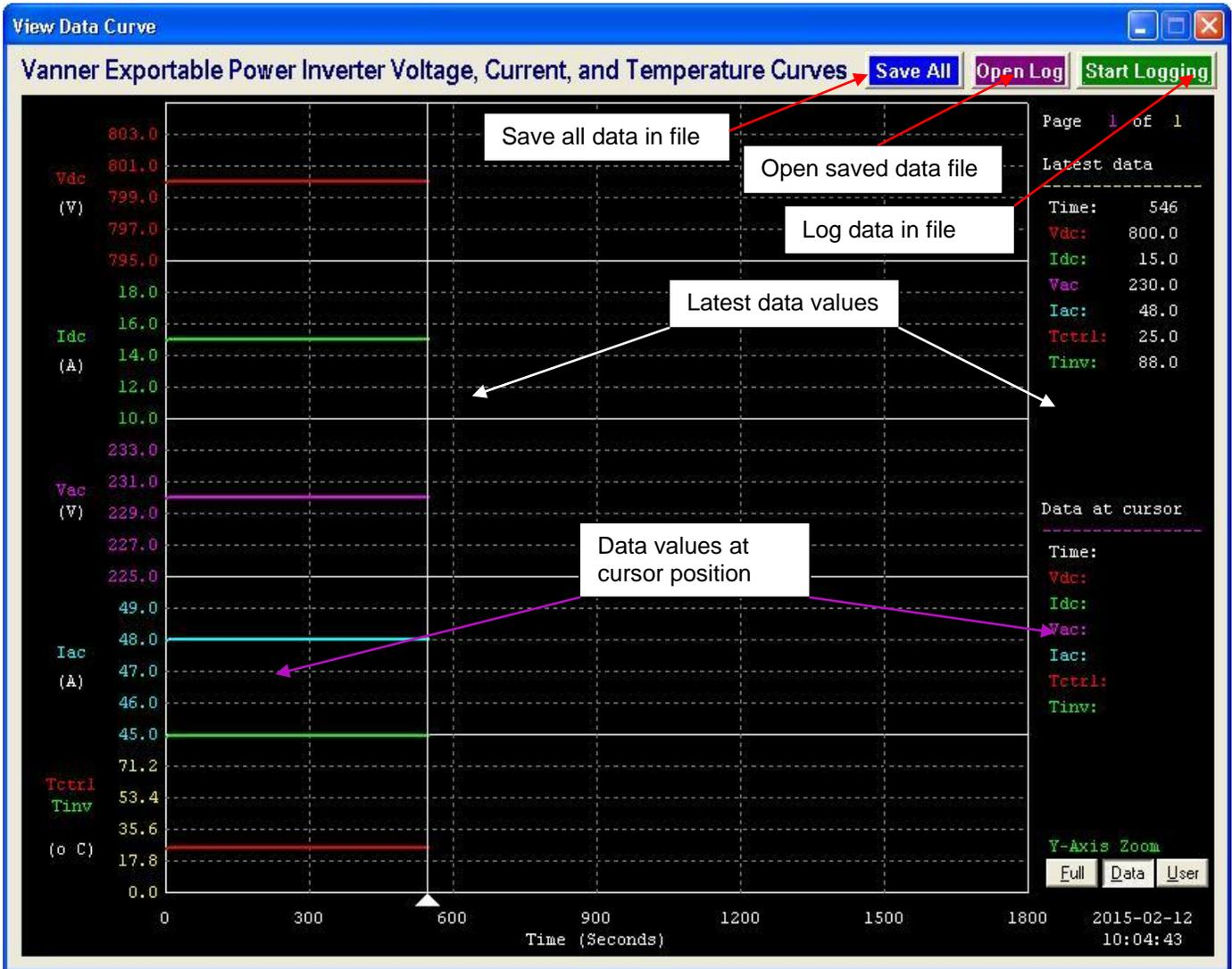
Figure 54. VEPI Data Curves Window – Real Time Data
