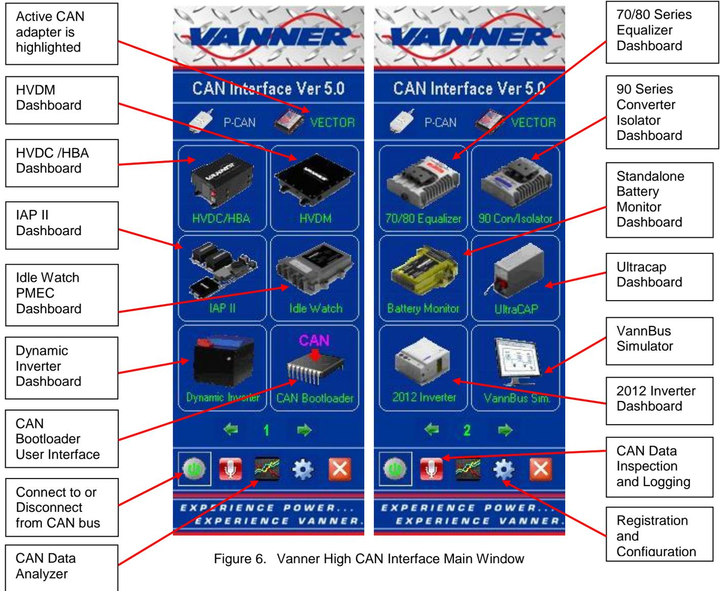
Figure 6. Vanner High CAN Interface Main Window
