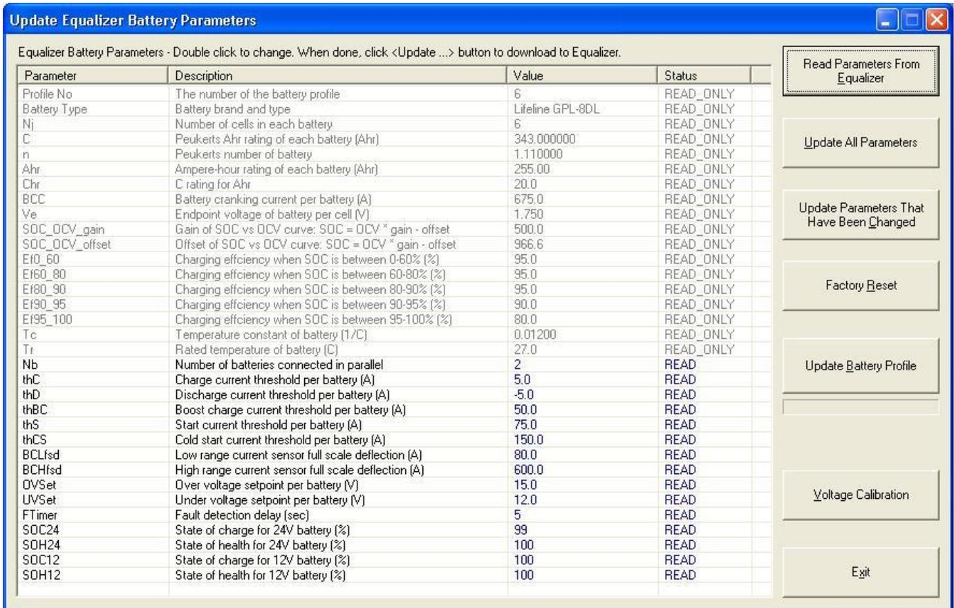
Figure 14. 70/80 Series Equalizer Battery Parameters Window
