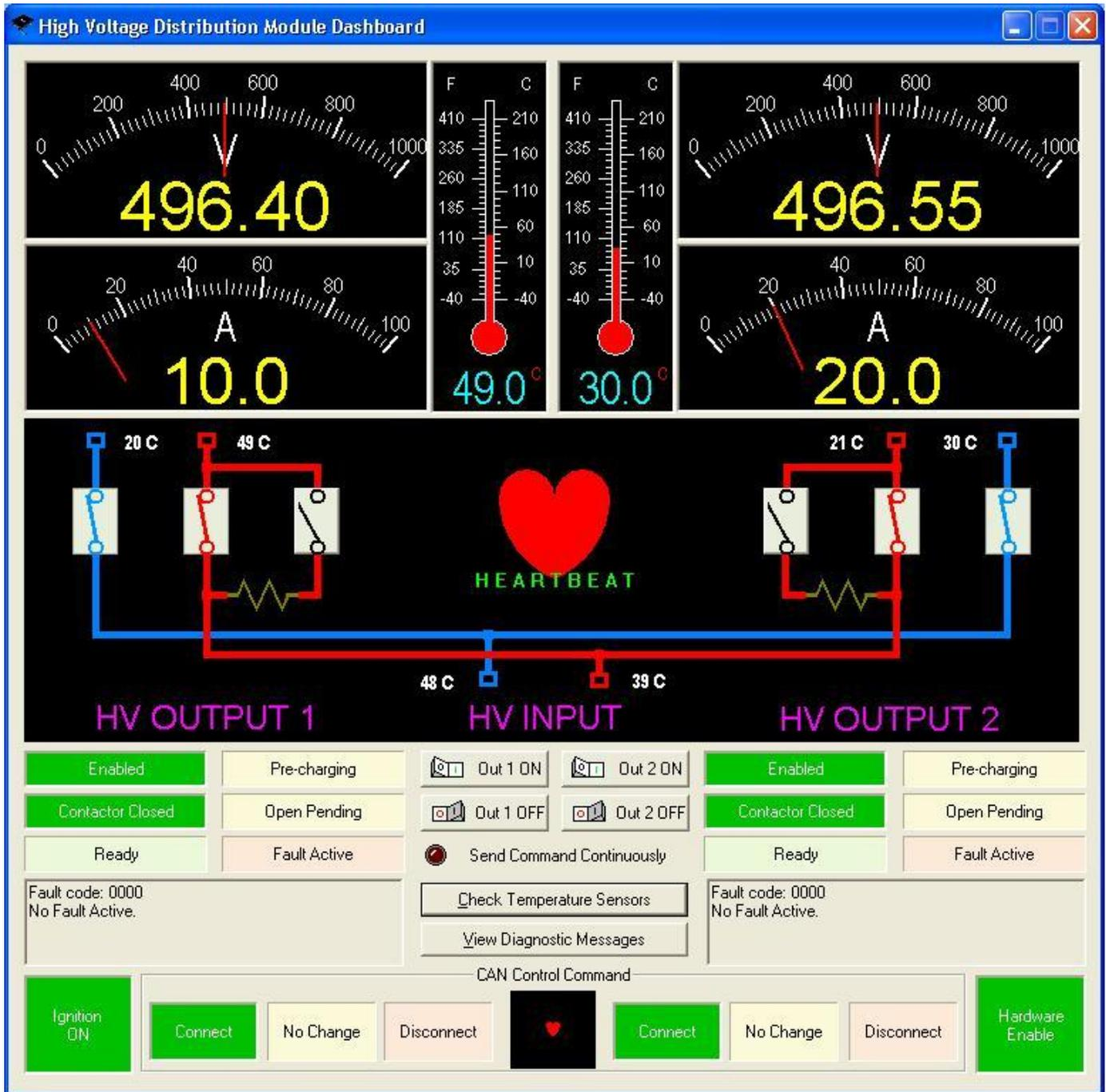
Figure 47. HVDM Dashboard with Temperature Values Displayed
