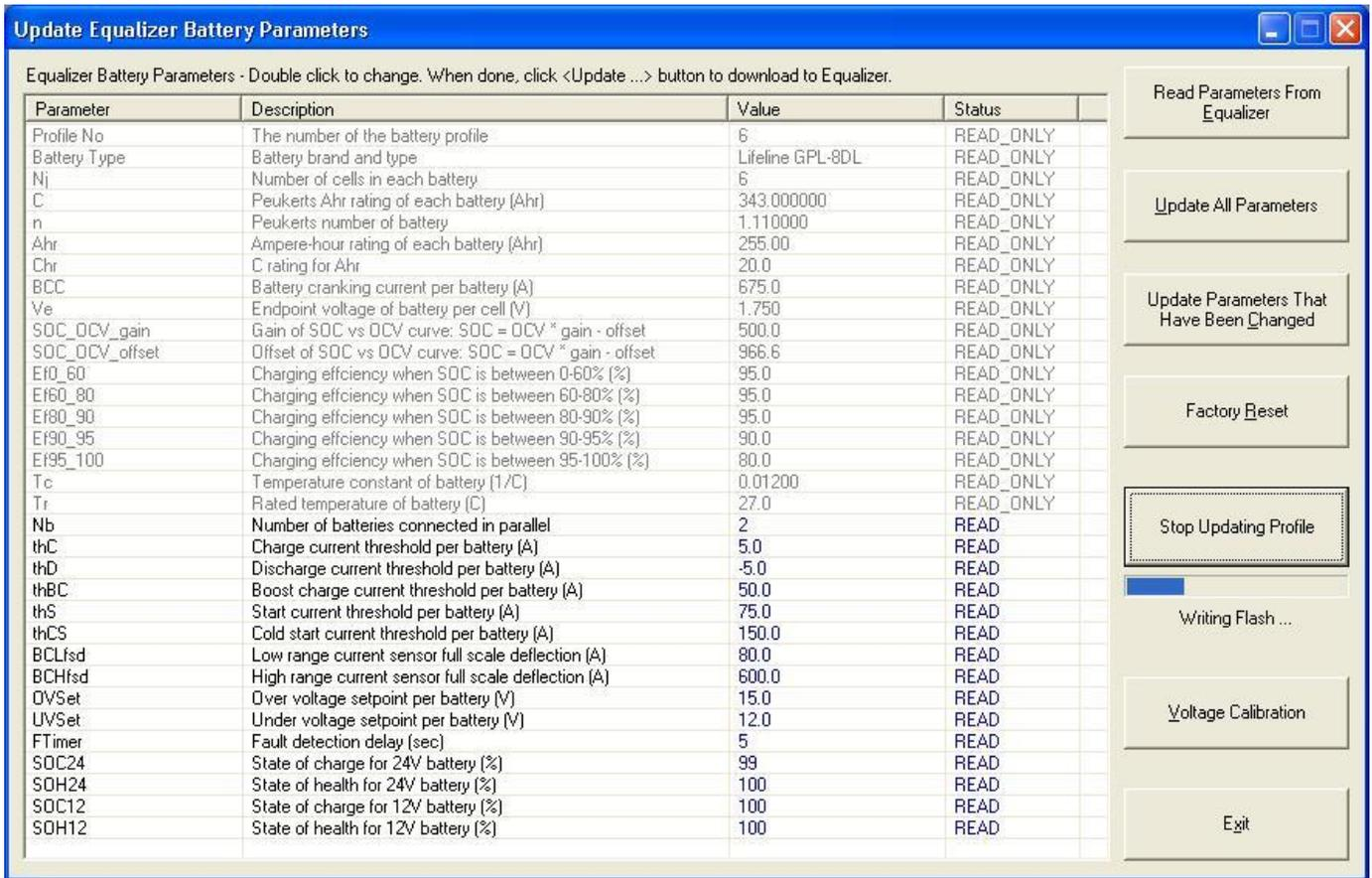
Figure 16. 70/80 Series Equalizer Battery Parameters Window – Update Battery Profile
