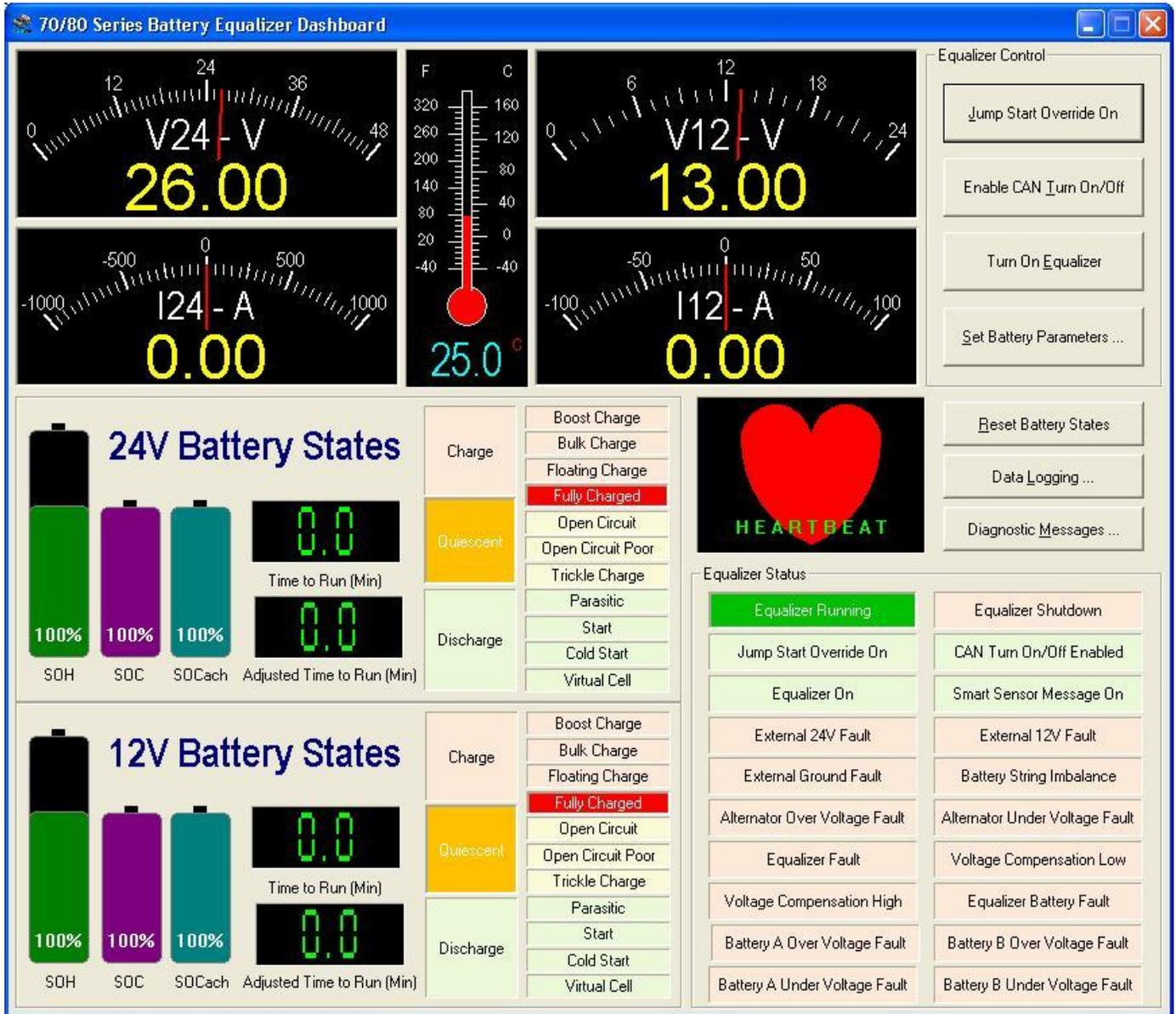
Figure 61. Equalizer Dashboard with VannBus Simulator Running
