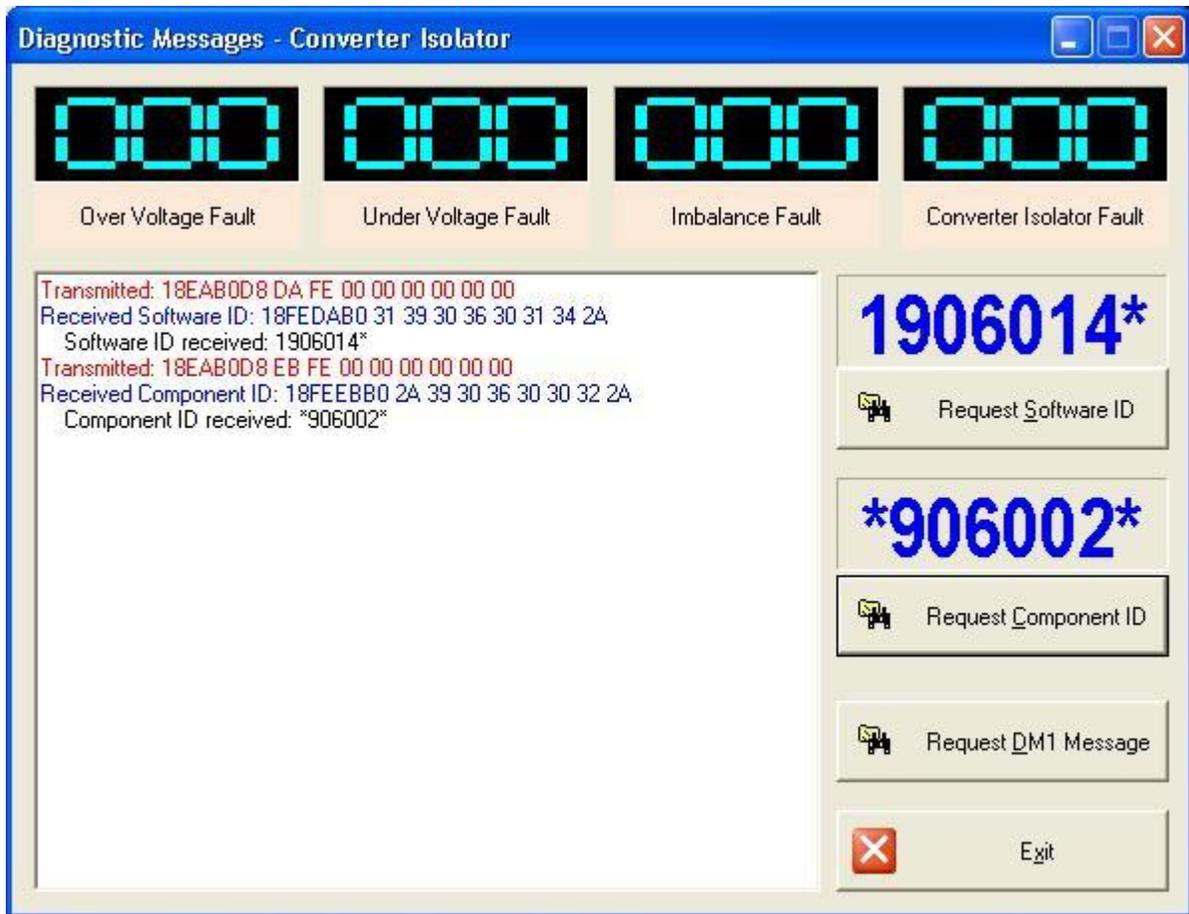
Figure 25. Converter Isolator Diagnostic Messages Window
