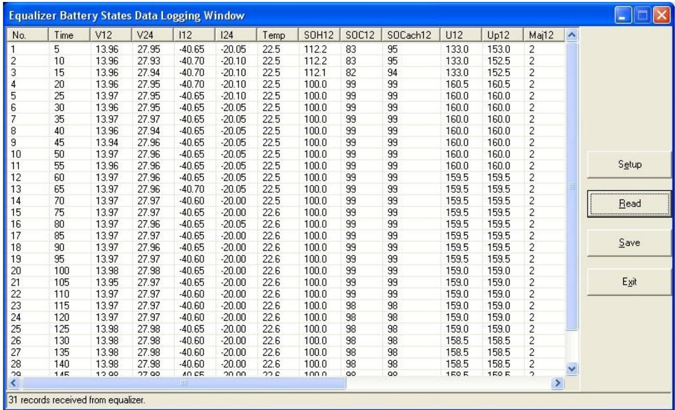
Figure 18. 70/80 Series Equalizer Battery States Data Logging Window
