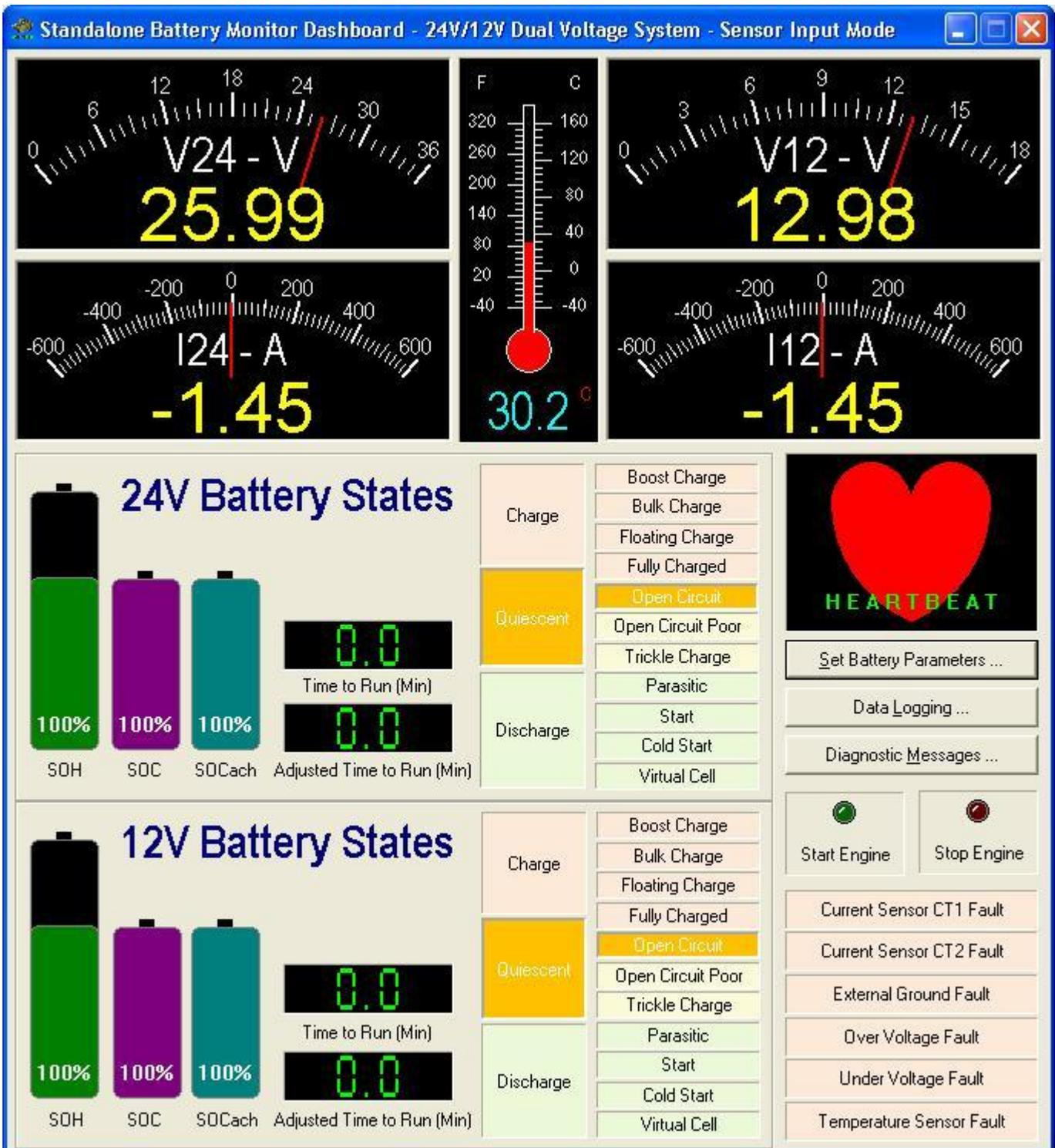
Figure 32. Standalone Battery Monitor Dashboard
