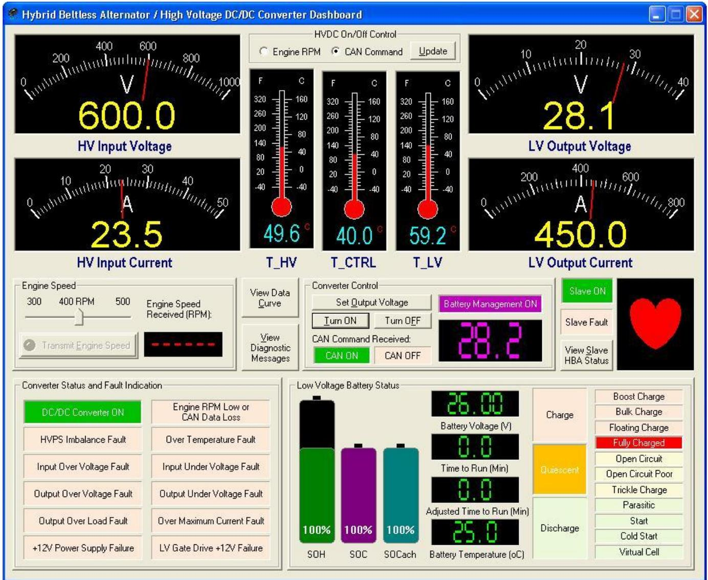
Figure 60. HBA Dashboard with VannBus Simulator Running
