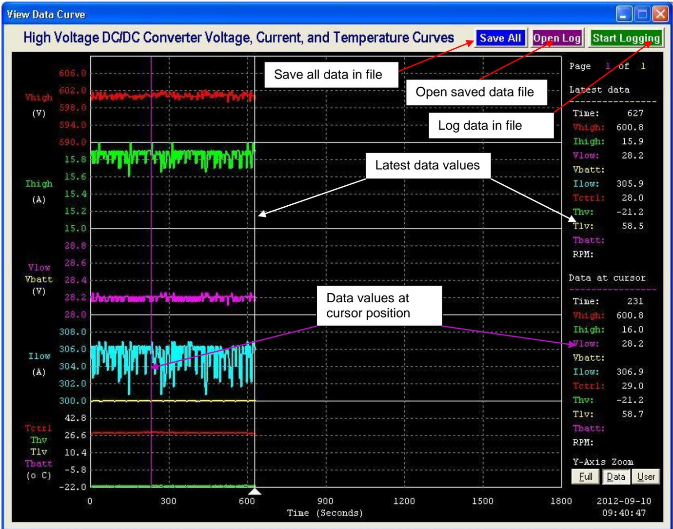
Figure 29. HVDC Data Curves Window – Real Time Data
