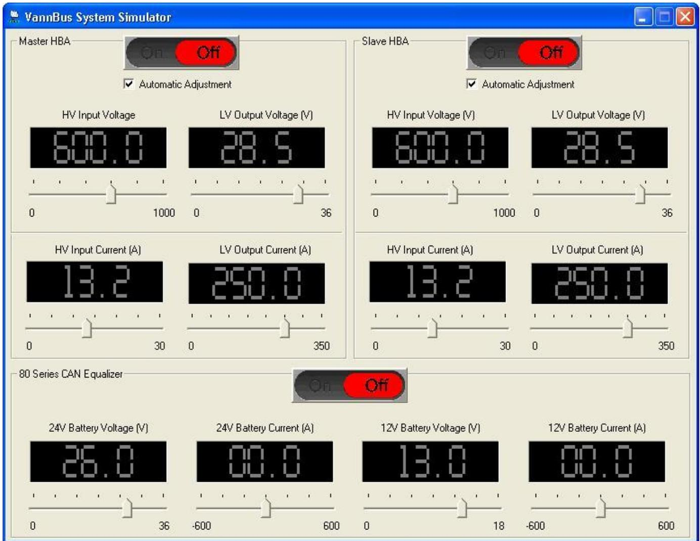
Figure 57. VannBus Simulator Main Window – OFF State
