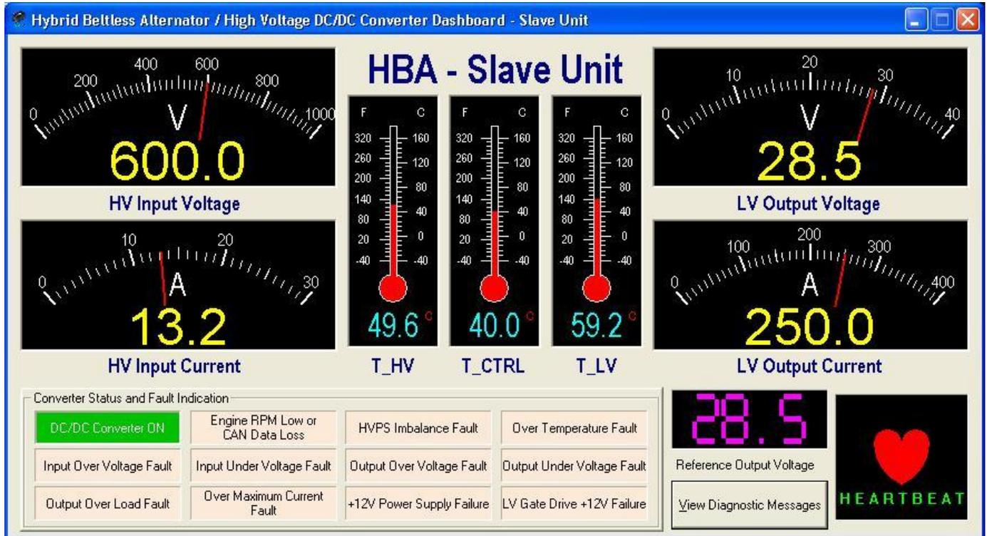
Figure 28. HVDC Dashboard – Slave Unit
