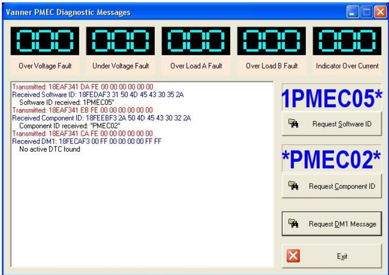
Figure 45. P MEC Diagnostic Messages Window
