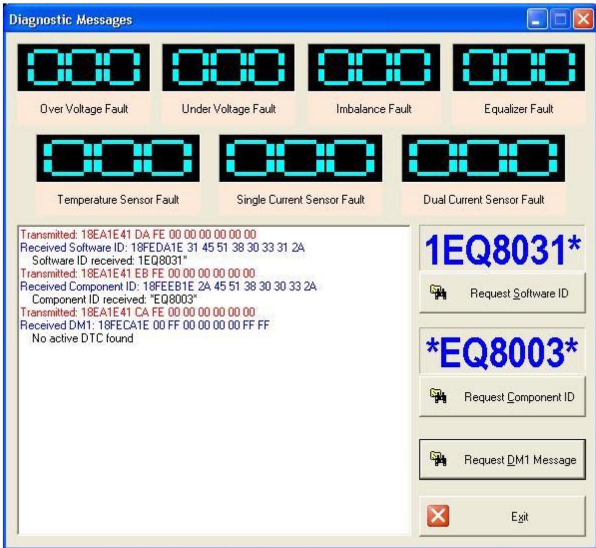
Figure 19. 70/80 Series Equalizer Diagnostic Messages Window
