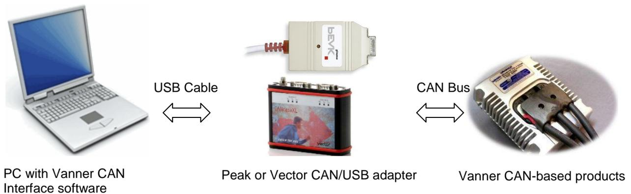
Figure 1. Vanner CAN Interface System Connection
